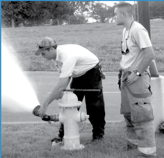
Justin Clemones, Compliance Specialist for Powdersville Water District, performs hydrant flow test while Jacob Pearson, from Powdersville Fire Department observes.
